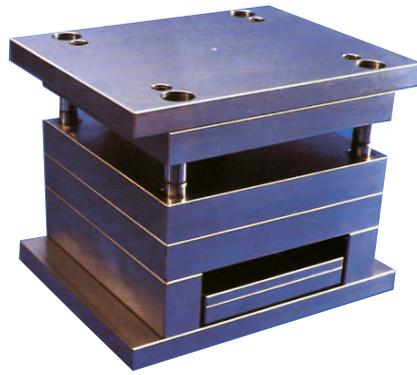
Undrilled precision ground plates
